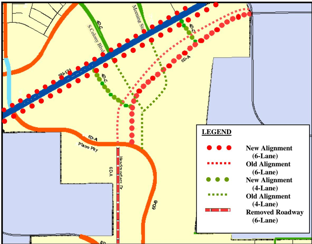
**Figure 5: Headquarters Drive Realignment and SH 121 EB Frontage Road Connectors**
